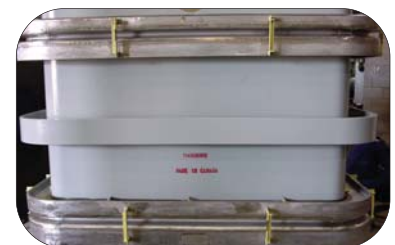
Containment passage rectangular expansion joints
