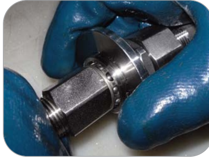
With sleeve retracted, pull nipple out
