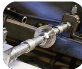
Hydrostatic test at 4000 psi
