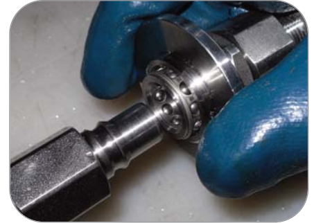
Fully disconnected in seconds
