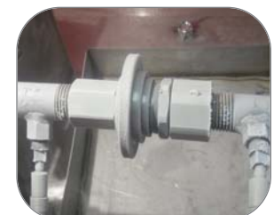
Liquid nitrogen test at -196°C
