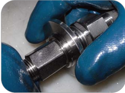
To disconnect, retract the sleeve
