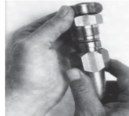
7- Tighten nut by hand before using wrench in final assembly.
