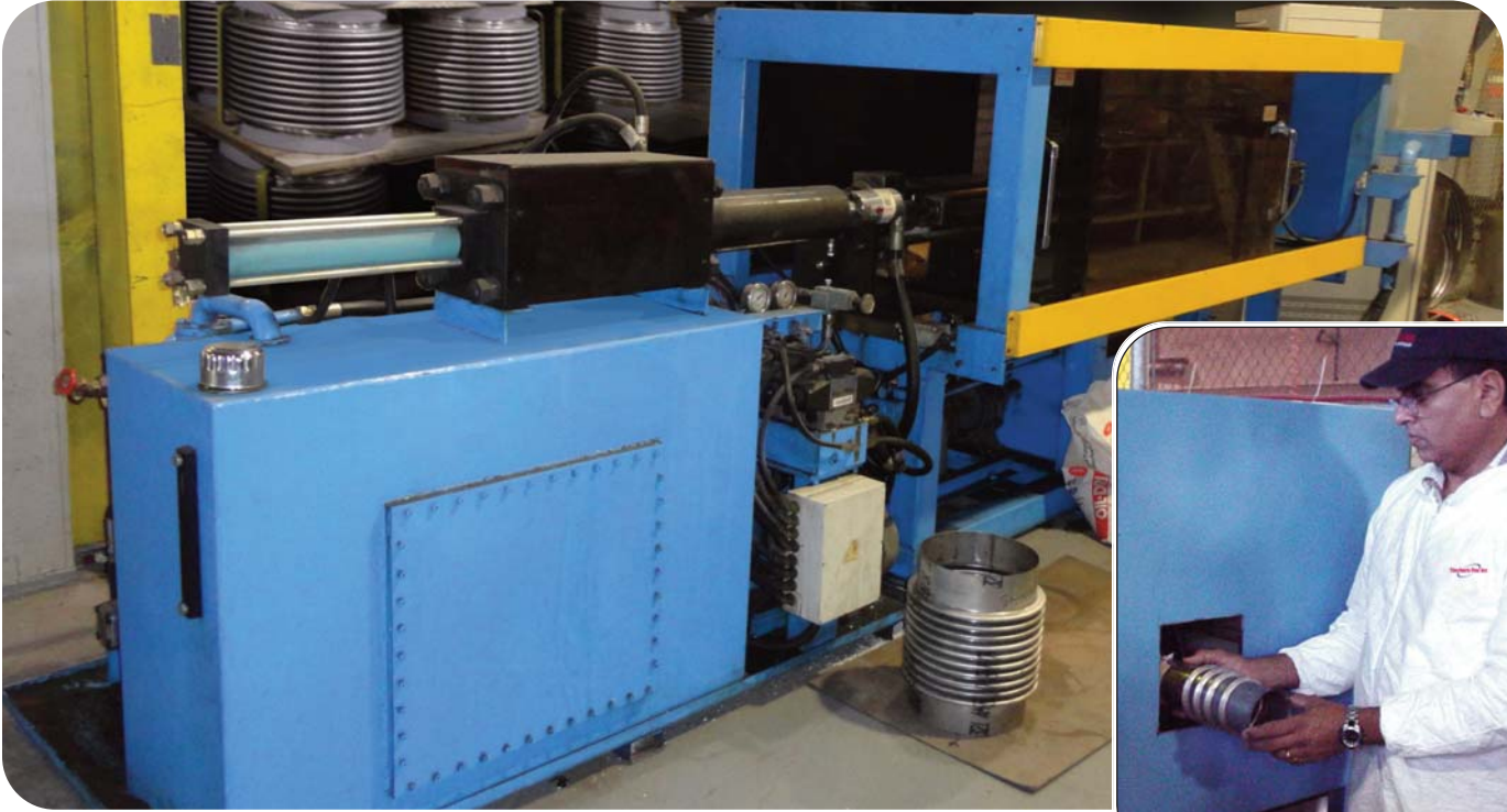
Thorburn's Precision hydro formed bellows manufactured with various ply thicknesses
