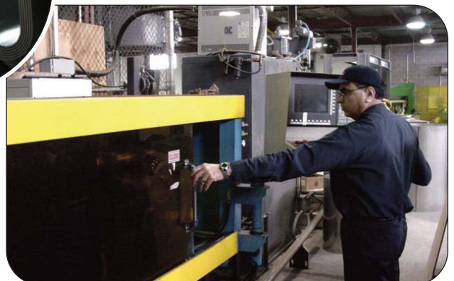
Thorburn's precision hydro forming bellows machine capable of forming from 10mm to 250mm
