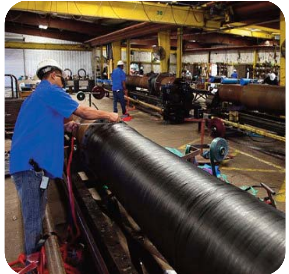
Custom hose building capabilities: 12mm to 1200mm Lengths: Up to 30m Design Pressures: Full vacuum up to 70 bar
