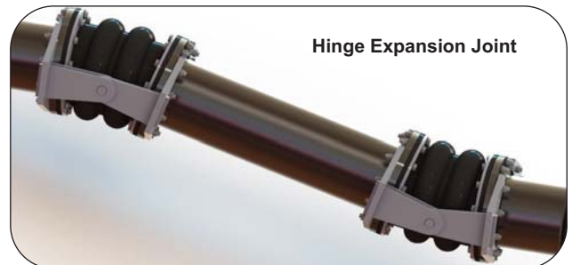
Thorburn's 42HP-6HU Universal Rubber Hinged Expansion Joint demonstrating the absorption of angular deflection in one plane
