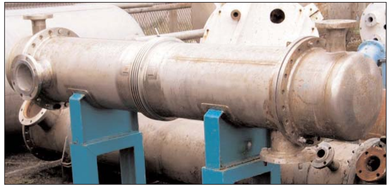
Thorburn's shell side heat exchanger bellows expansion joints are most commonly found on T.E.M.A., AEM, BEM and NEN fixed tubesheet heat exchangers such as the one shown above. Thorburn can also provide tube side heat exchanger expansion joints for customized floating head heat exchangers e.g. AET & BET configurations which are specially designed to resist both the internal pressure from the tube side as well as the external pressure buckling loads from the shell side.
