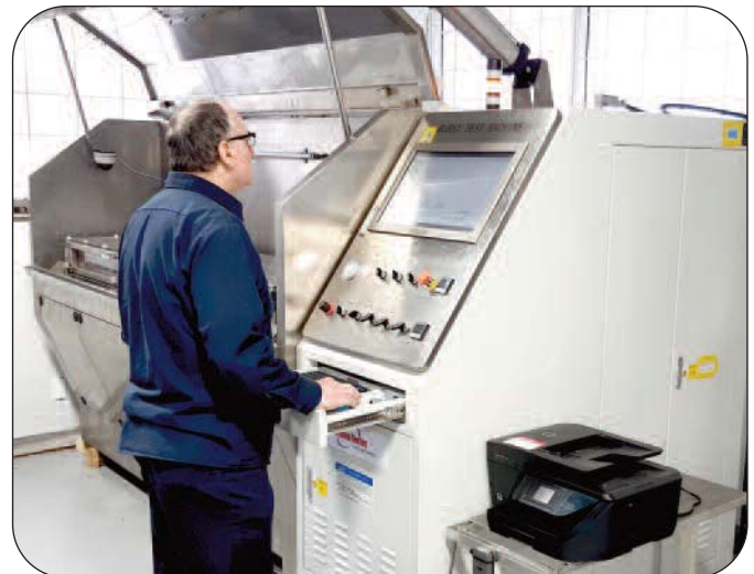
Thorburn burst testing capabilities up to 4000 BAR
