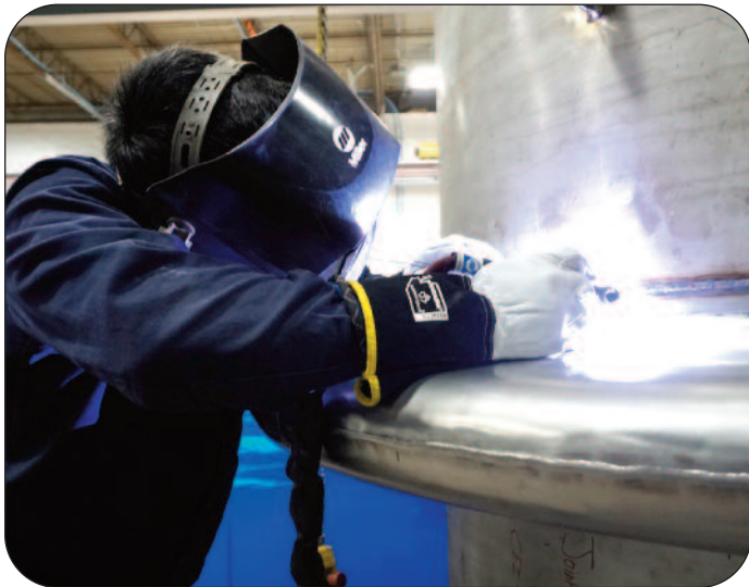
Welding a Thorburn Series AFS single convolution lens High-Core bellows
