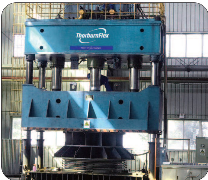
Thorburn's large hydroforming press making large multi-convolutions up to 4 meters with convolution heights up to 250mm (10 inches)
