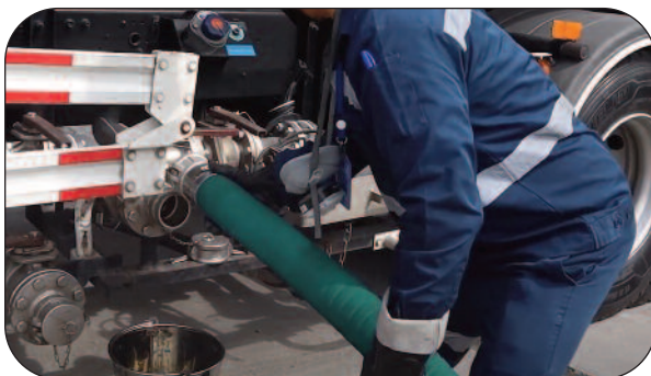
Hose Assemblies are made with UHMWPE, XLPE, PTFE, FEP, EPDM, CSM & FKM Materials
