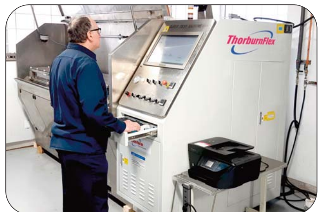
Hose Assembly Burst Testing (up to 4000 bar)
