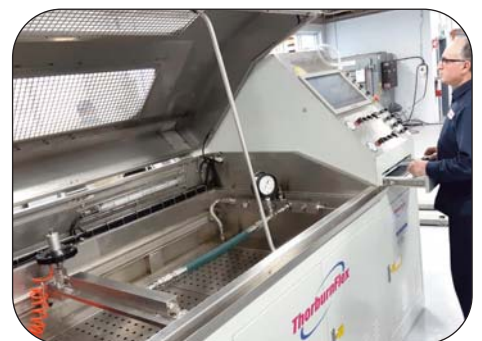
Hose Assembly Proof Testing up to 1000 bar
