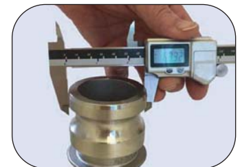
Measuring OD of adapter
