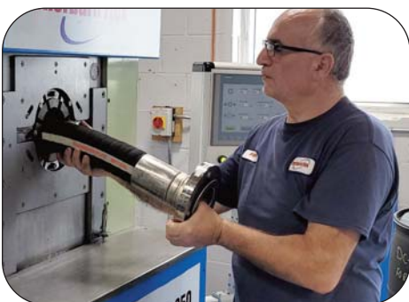
Fitting To End Joint Crimping Process
