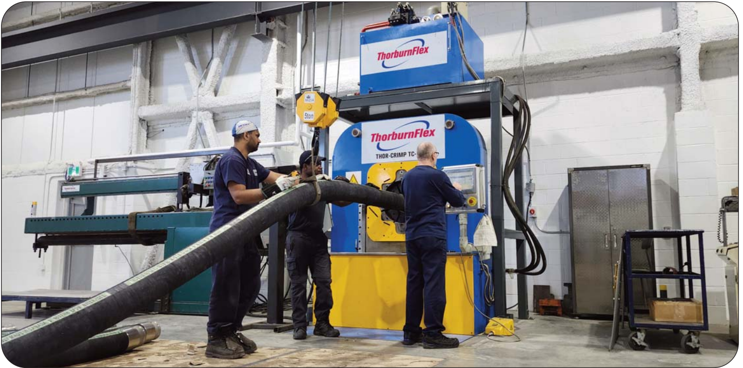
DN 3 (1/8") to DN600 (24") Crimper, largest in the world - more than 3 million lbf (1.5 million kgf)
