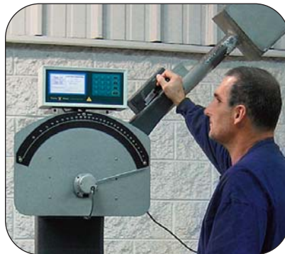
Charpy V notch impact testing on sheet metal
