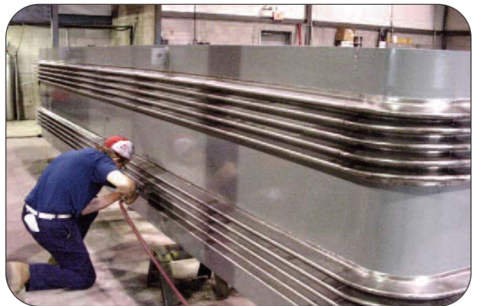
Thorburn Duct Flex™ 316SS round corner expansion joint for use on a power plant steam generator
