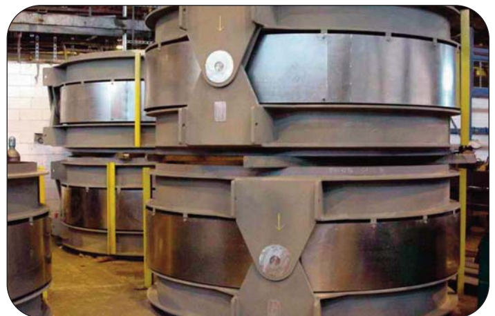
Thorburn's ASME Section III class 2 hinged expansion joints were installed at the qinshan PHWR nuclear reactor's dousing system
