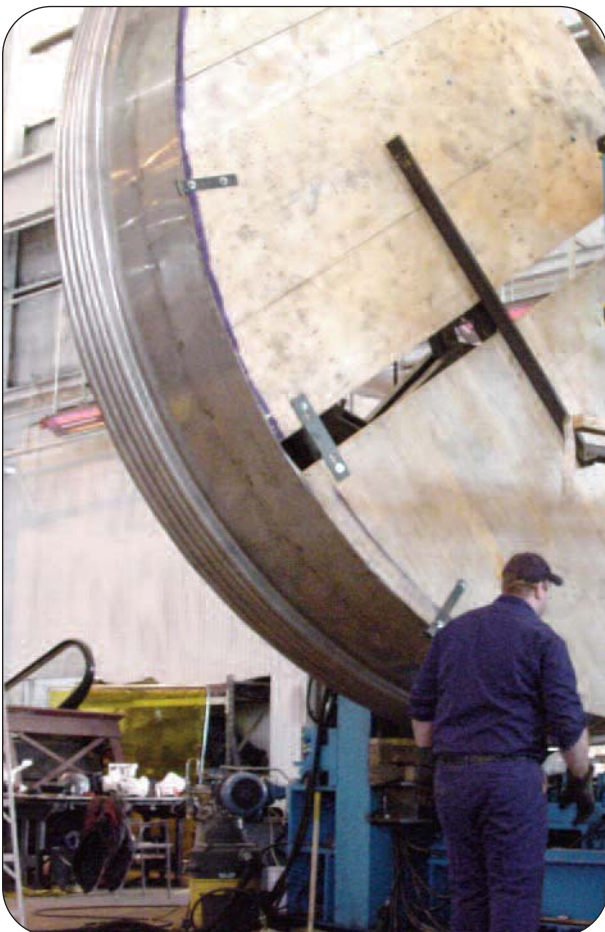
Thorburn Duct Flex™ Series SDF 22 ft (6.7 m) diameter expansion joint bellows for the Tuxpan combined cycle power plant located in Veracruz, Mexico
