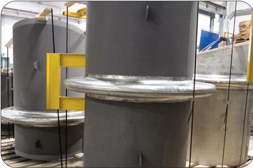
Thorburn Series AFS High-Core bellows expansion joints ready for shipping
