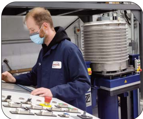
Mechanical forming metal tubes into bellows from sizes 50mm to over 4m
