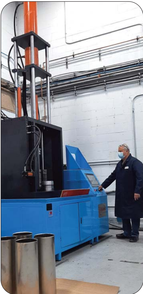
Thorburn hydroforming bellows (all convolutions simultaneously)
