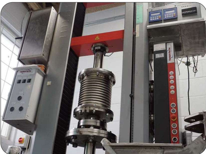
Metal bellows cyclic fatigue testing
