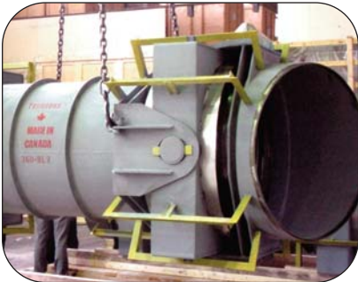
MAIN STEAM LINES Gimbal Steam Penetration Expansion Joint
