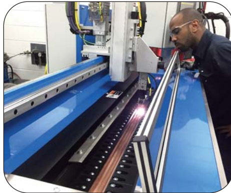
Robotic fusion seam welding metal sheets into tubes with ASME Section II, 2014/68/EU PED materials conforming to ASME Section III Design
