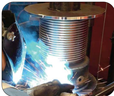
Welding flanges to bellows to ASME sections III, VIII, IX and PED procedures
