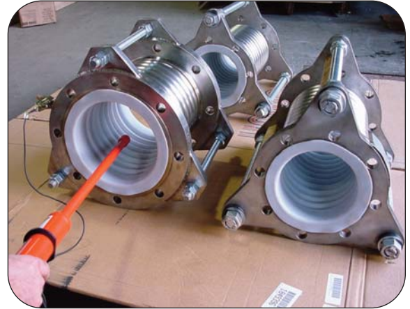
Hot-Flex expansion joint PTFE liner undergoing a 10,000 Volt spark test to detect pin holes
