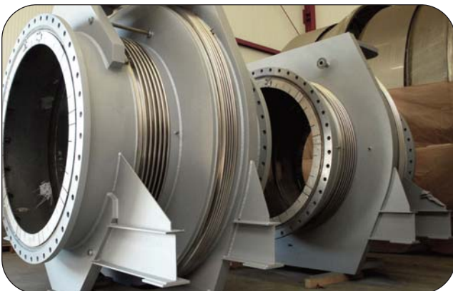
FCCU pressure balanced expansion joint
