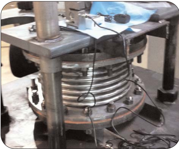
Thorburn's Model RLB-SF Cyclic Movement Testing
