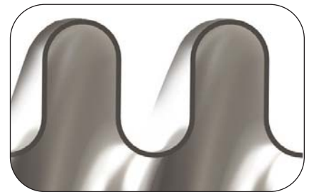
Convolution shape before deflecting. When the bellows compresses, the side walls bend to shorten the bellows
