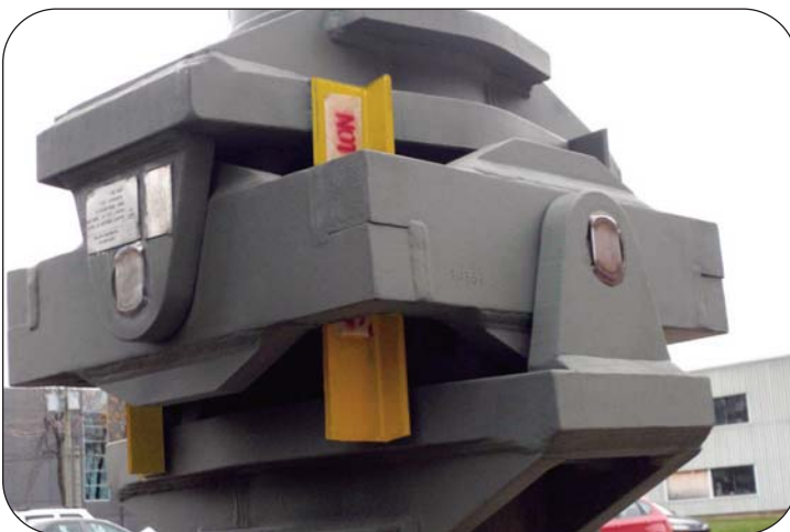
Final assembly of a Thorburn Single Flex™ Series GF large diameter, Ultra High Pressure (300mm10,000 Kpa Design / 15,000 Kpa), expansion joint ready for crating and shipping
