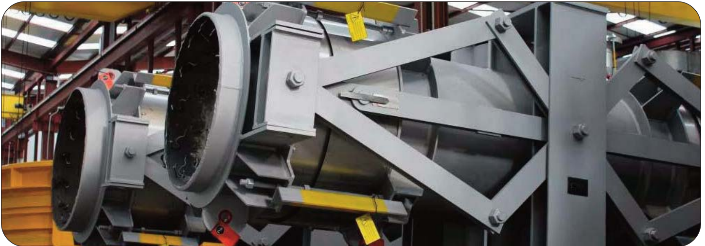
FCCU high temperature expansion joint with pantograph linkages
