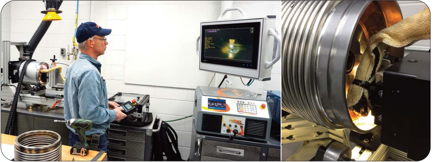
Thorburn automatic circumferential micro GTAW/PAW welding
