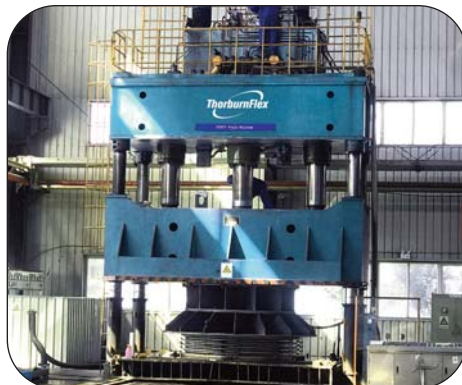
Hydro-forming metal tubes into bellows from sizes 25mm to over 4m
