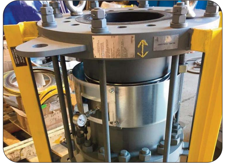
Thorburn's Dual Flex Model RLB-DFT - Tied Universal Rubber Lined Metallic Expansion Joint System for the SUNCOR Fort Hills Project. Design pressure 35 bar (550 psi) test pressure 53 bar (800 psi)
