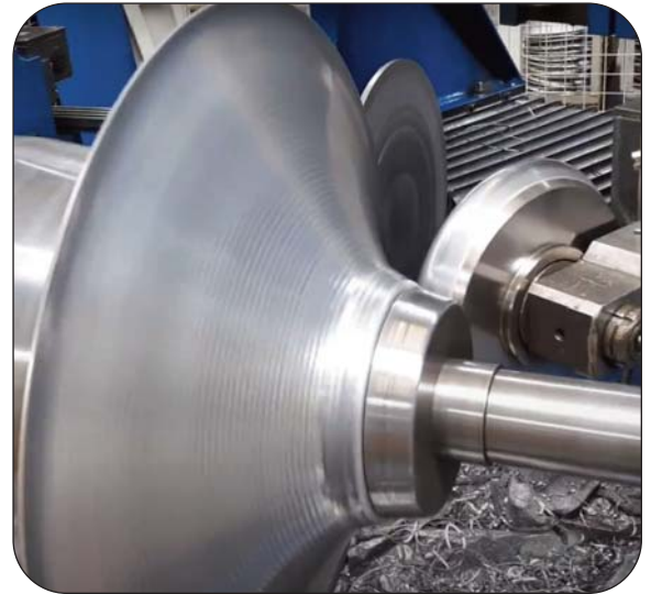
Bellows spinning machine forming a Thorburn lens style bellows
