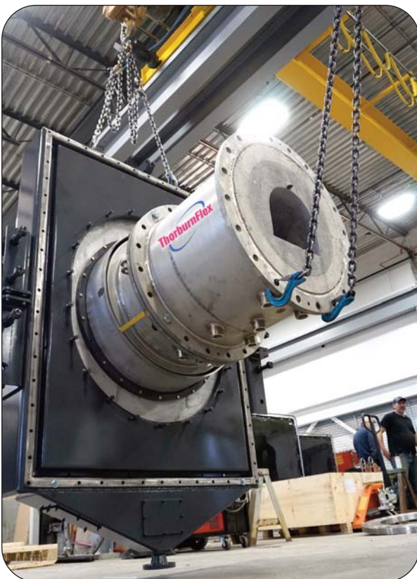
Thorburn Series BT-CFB bed transfer expansion joint ready for inspection
