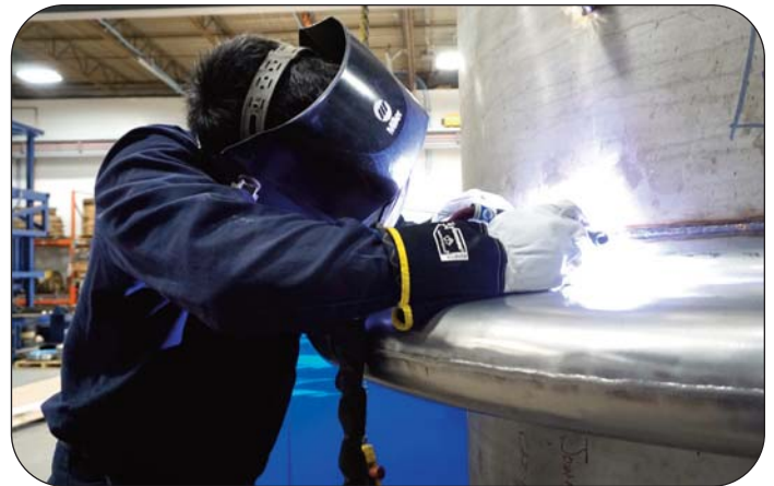
Welding a Thorburn Series AFS single convolution lens High-Core bellows
