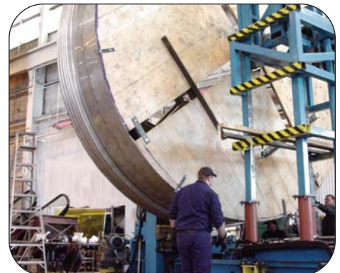
Roll forming metal tubes into large diameter bellows up to 10m in size
