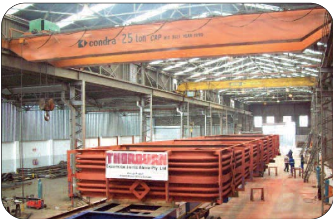
Duct Flex™ round corner expansion joints at Thorburn's workshop in Johannesburg South Africa
