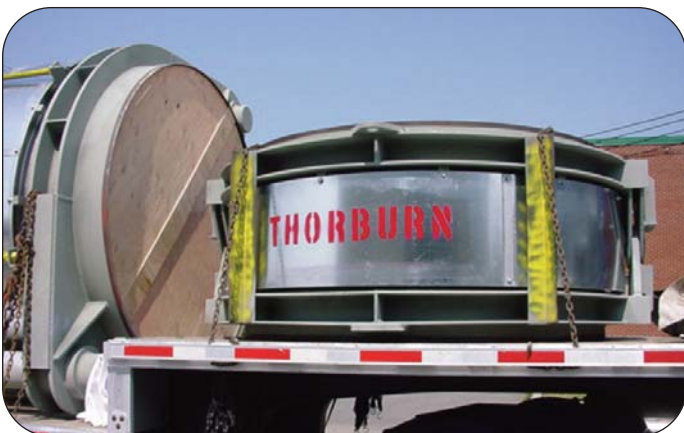
Thorburn DFT tied universal and hinged expansion joints for a biomass power plant
