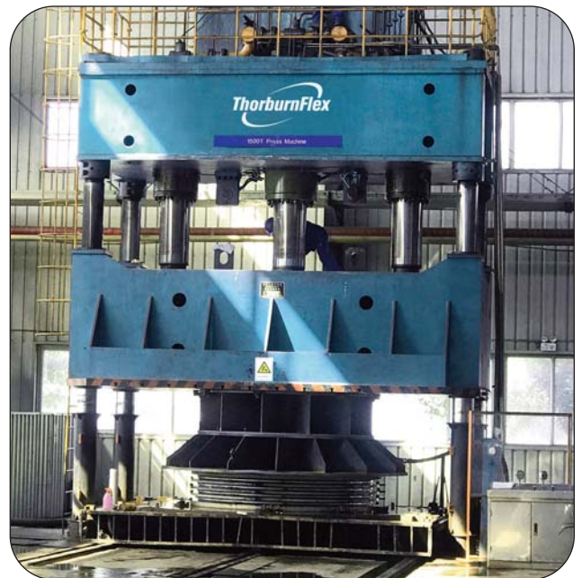
Thorburn's large hydroforming press making large multi-convolutions up to 4 meters with convolution heights up to 250mm (10 inches)
