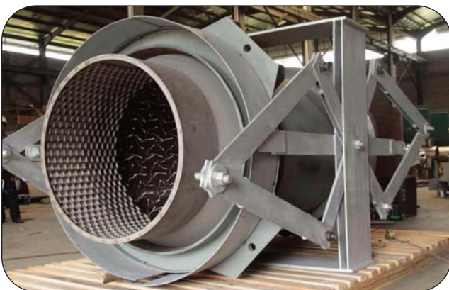
Thorburn FCCU hot wall expansion joint with a gimbal ring that permits lateral deflection in two planes and a pantographic linkages that equalizes the amount of axial compression that each bellows will absorb
