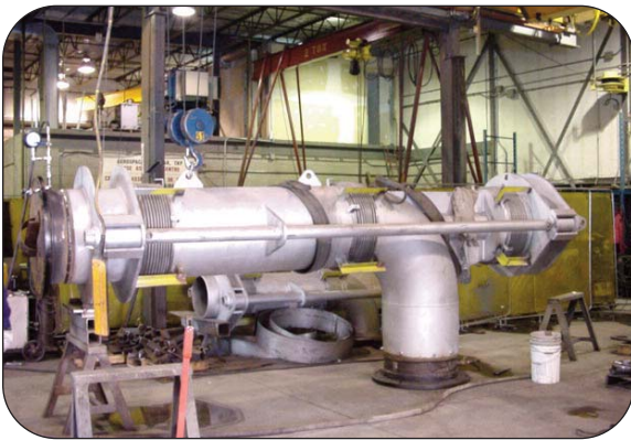
A Boiler Feed Pump provides high pressure water to the boiler which in turn produces steam to drive the steam turbine
