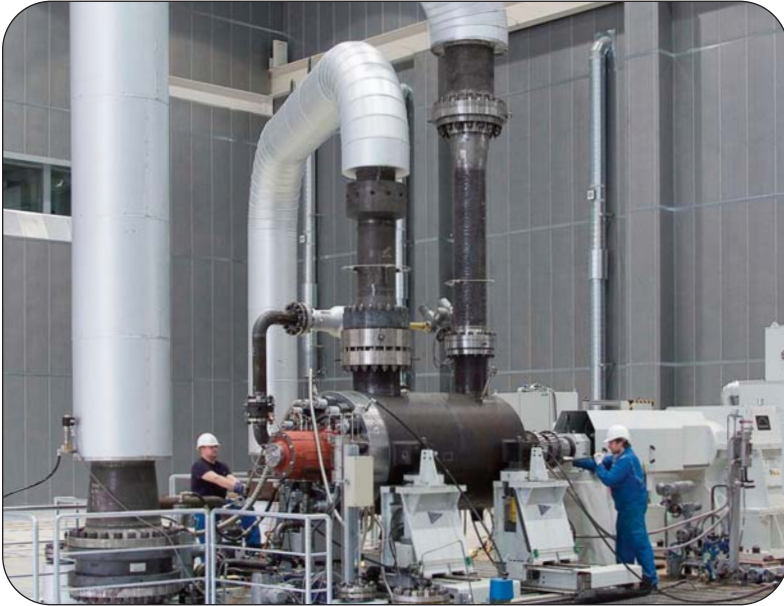
A Boiler Feed Pump provides high pressure water to the boiler which in turn produces steam to drive the steam turbine
