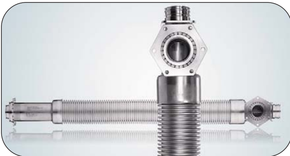
Bellows for trim tank kerosene lines connects the rigid transfer pipe to the flexible trim tank in the horizontal stabilizer and enables continuous drainage and leakage detection for the inner fuel line
