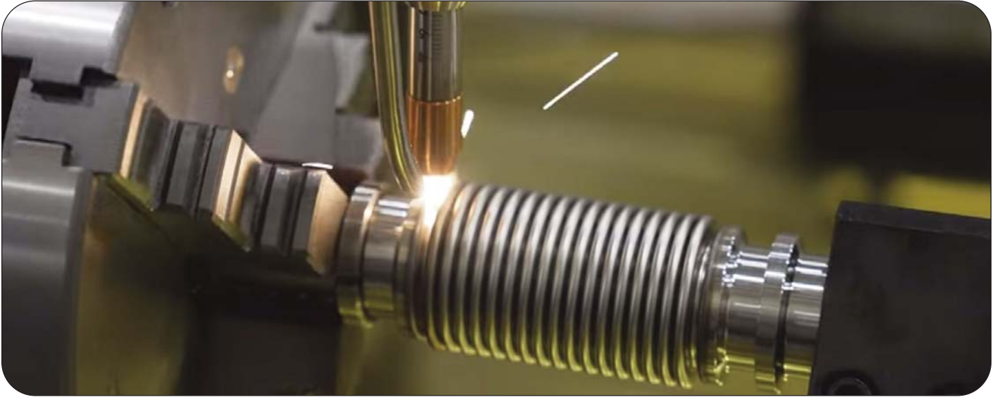
Thorburn's external automatic micro GTAW/PAW robotic welding
