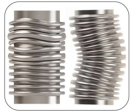
In-plane instability | Column instability
