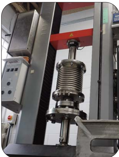
Metal bellows cyclic fatigue testing
