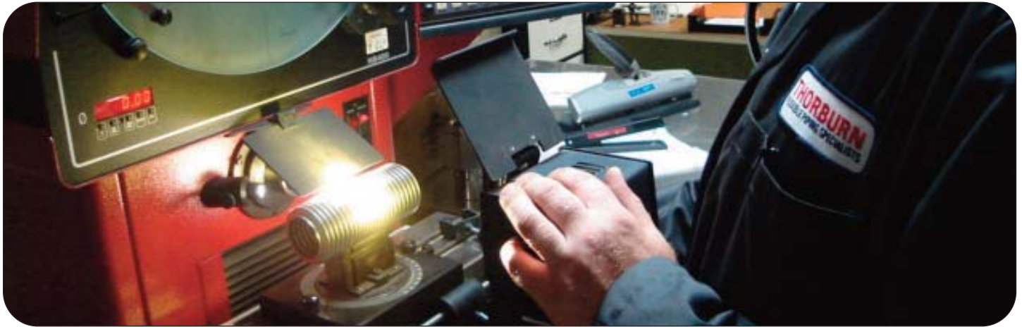
Inspecting bellows using an optical comparator to check dimensional accuracy and surface defects
