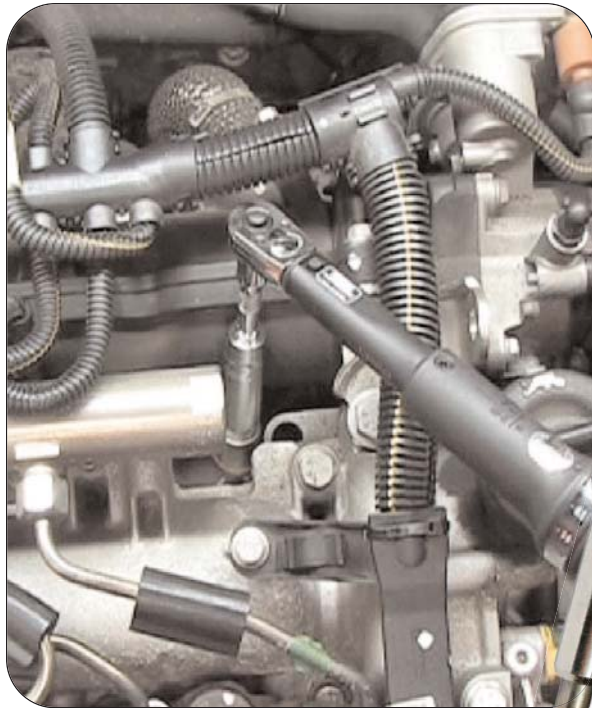
Installed pressure sensor glow plug assembly
