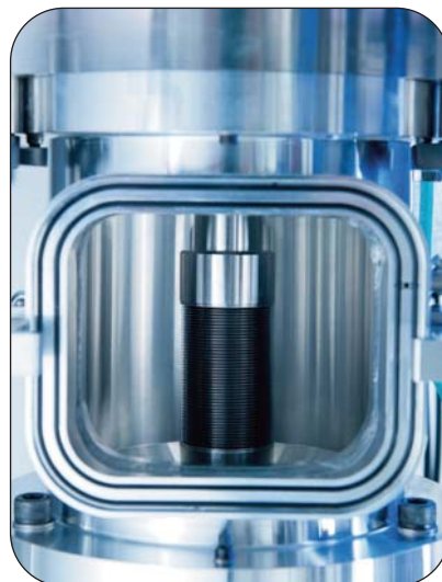
Helium leak testing metal bellows
