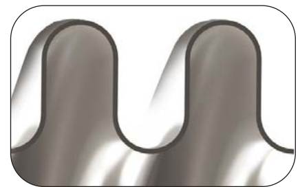
Convolution shape before deflecting. When the bellows compresses, the side walls bend to shorten the bellows
