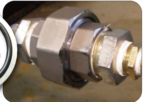
The same union with Thorburn Retrofit Seal installed (Not leaking when hand tightened to 5500 psi / 367 bar)
