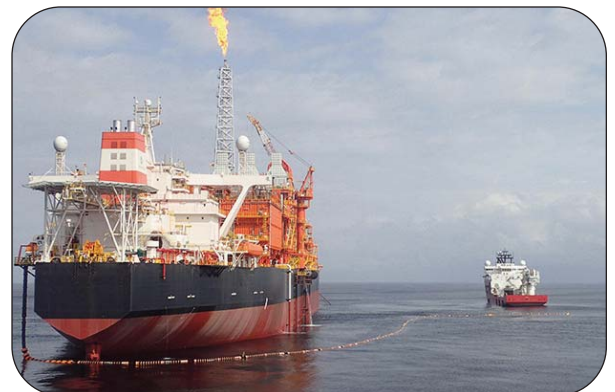
Tandem Cargo Offloading - Mooring System
