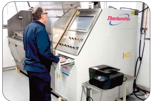
Hose Assembly Burst Testing (up to 4000 bar)
