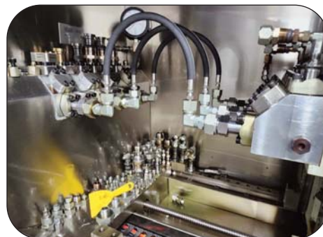
Hose Assembly Impulse Testing (@ 150°C up to 1000 bar)
