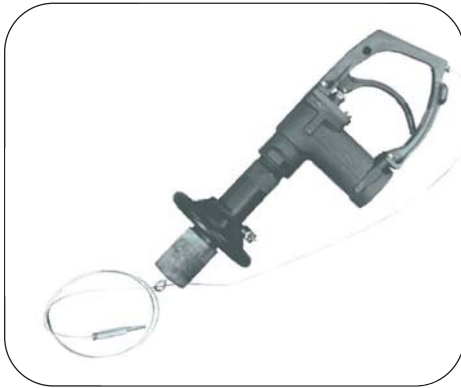
A | Over Wing Fuel Nozzle Body: Cast aluminum Main Stem: Stainless steel Stem Seal: Buna-N O-Ring Disc: Viton® (FKM) Sizes: 1 1/2"
