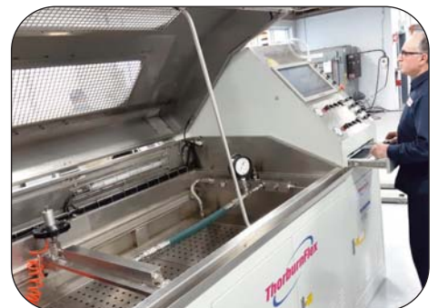
Hose Assembly Proof Testing up to 1000 bar
