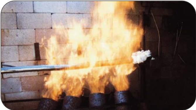
Thorburn's Ball Joint Armor-Flex™ tested at 1100°C
