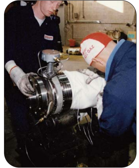
Installing inner insulation on Sure-Temp™ hose
