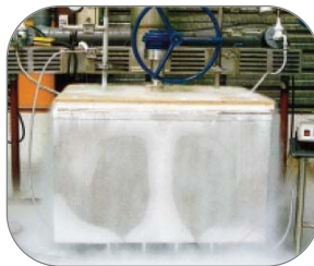
Cryogenic test bench at -320°F
