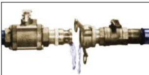
Ordinary Ball Valves Added = Spillage
