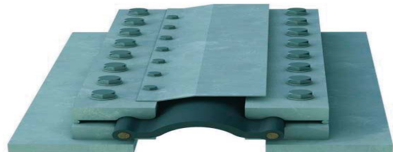
Thorburn's Dog-Bone Expansion Joint Model DBE-CR with flexible element, clamping bars and bolt-in liner
