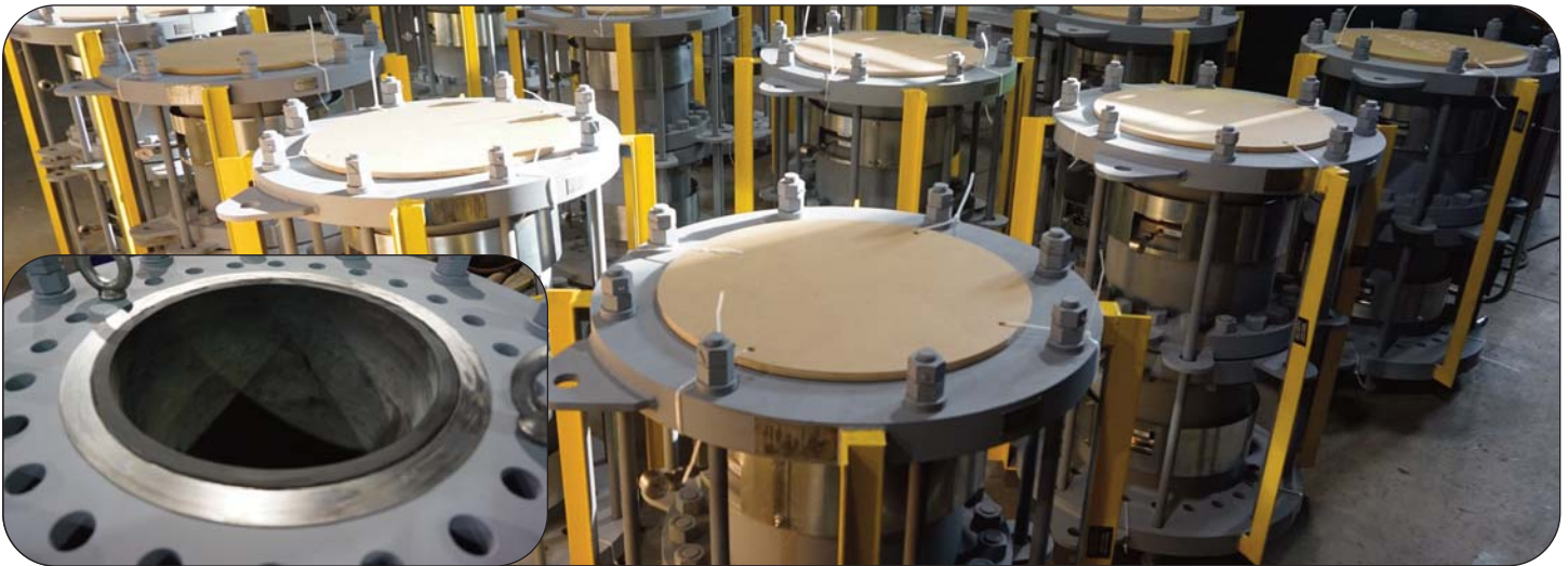
Thorburn's Dual Flex Model RLB-DFT - Tied Universal Rubber Lined Metallic Expansion Joint System for the SUNCOR fort Hills Project. Design pressure 35 bar (550 psi) test pressure 53 bar (800 psi)
