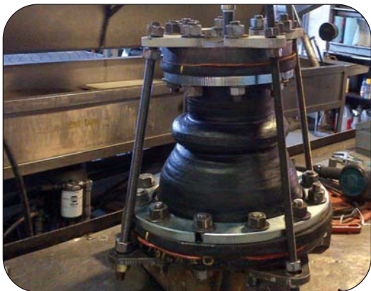
Thorburn's 42HP-CR Concentric reducer 300mm (12") by 125mm (5") ID tested at 16 bar
