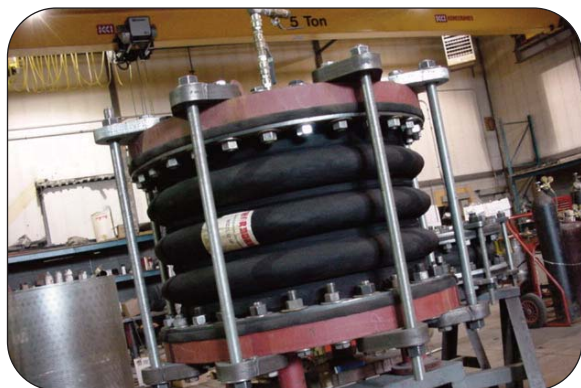
Thorburn's Model 42HP-HDX being assembled, ready for external testing. Thorburn proprietary system was successfully tested in a pressure chamber to 225 psi (1550 kPa) external pressure.
