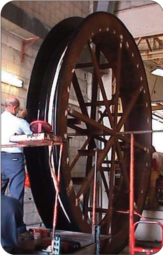
Thorburn's rubber pressure piping expansion joints are hand crafted by skilled technicians using the most advanced elastomers, calendared fabrics and metallic reinforcements. Sizes from 25mm (1") up to 3600mm (144") with design pressures up to 20 bar with 4 to 1 safety factor
