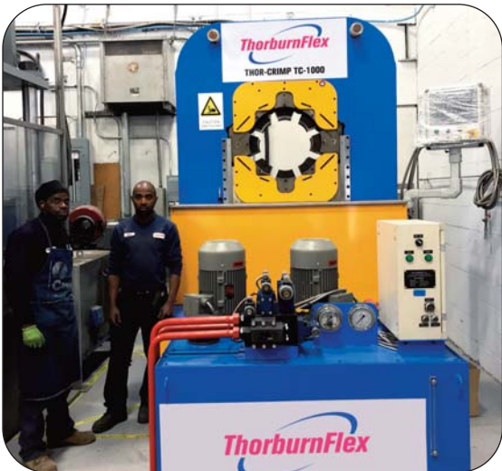
Thorburn possesses one of the world's largest crimping machines with a 1000 ton crimping force & 590mm jaw opening
