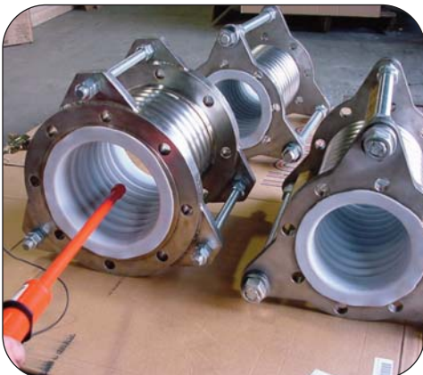
Hot-Flex expansion joint PTFE liner undergoing a 10,000 Volt spark test to detect pin holes
