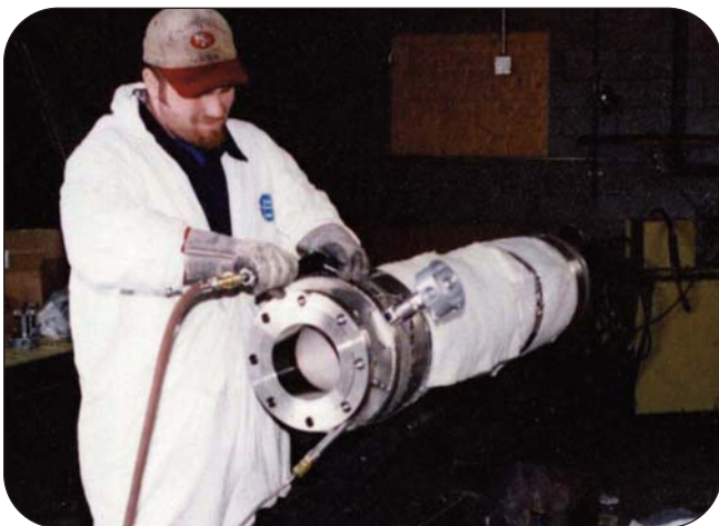
Performing quality check of Sure-Temp™ hose
