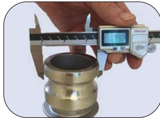
Measuring OD of adapter
