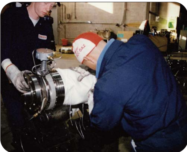
Installing inner insulation on Sure-Temp™ hose
