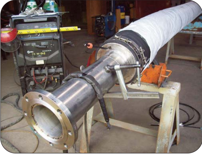
Manufacturing Sure-Temp™ electrically heated hose assembly
