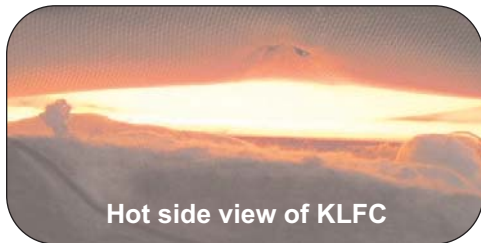
Hot surface performance test for 96 hours @ 2000°F (1094°C) as per ASTM C-411
