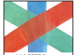
M12 PTFE films are crossed & laminated to produce a Multi-Directional based corrosion barrier
