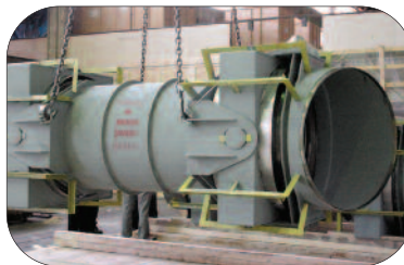
Main steam penetration gimbal expansion joints
