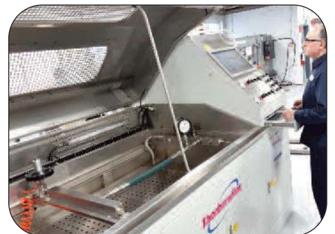
Hose Assembly Proof Testing up to 1000 bar
