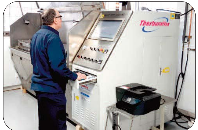
Hose Assembly Burst Testing (up to 4000 bar)
