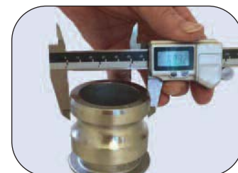
Measuring OD of adapter
