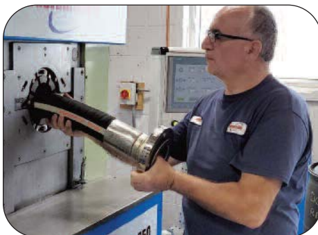
Fitting to End Joint Crimping Process
