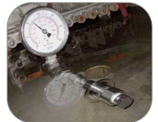
Pneumatic test at 100 psi
