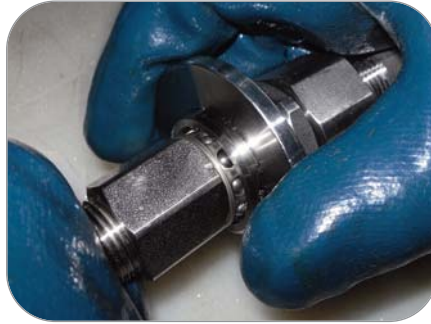
With sleeve retracted, pull nipple out
