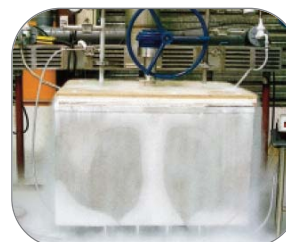
Cryogenic test bench at -320°F
