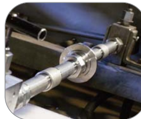
Hydrostatic test at 4000 psi
