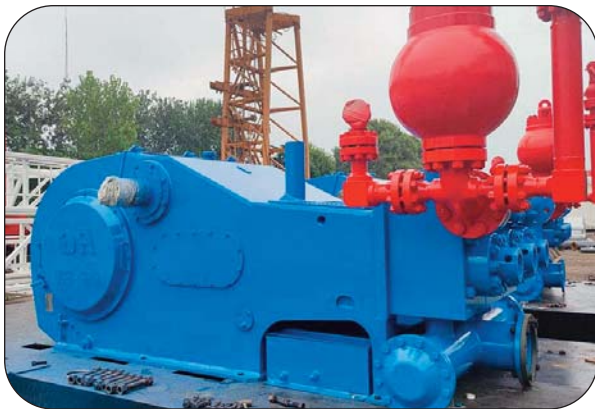
Mud Pump Suction & Discharge
