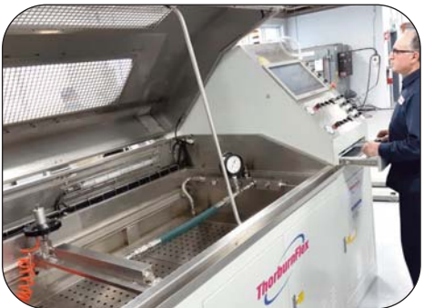
Hose Assembly Proof Testing up to 1000 bar
