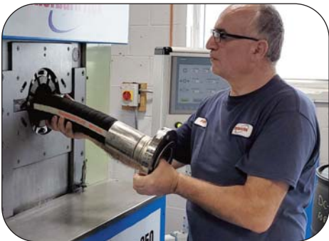
Fitting To End Joint Crimping Process
