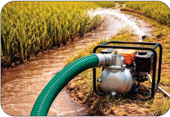
Pump suction and discharge
