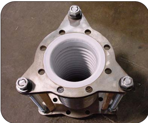
Thorburn's Hot-Flex with isostatically molded unpigmented PTFE convolutions
