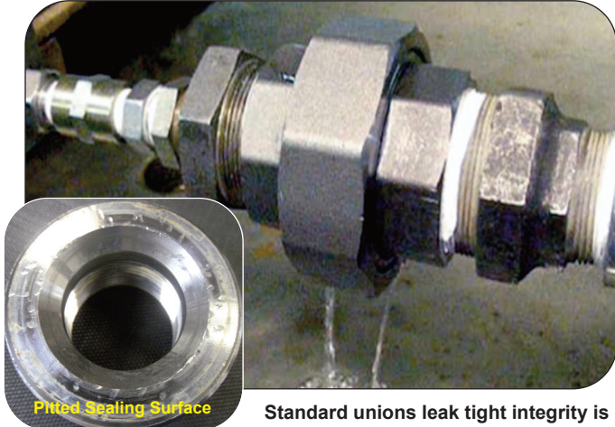
50mm/2 inch threaded leaking at 0 psi / 0 bar
