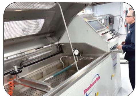
Hose Assembly Proof Testing up to 1000 bar
