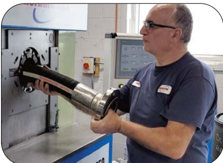
Fitting to End Joint Crimping Process
