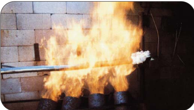
Thorburn's Ball Joint Armor-Flex™ tested at 1100°C
