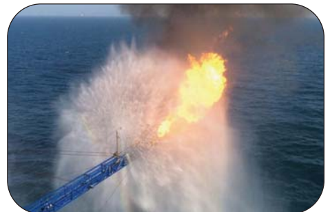
Rig Cooling & Fire Suppression
