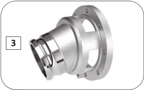
Adapter - API to 4" drop adapter nitrile seal, two piece design with sight glass
