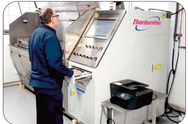
Hose Assembly Burst Testing (up to 4000 bar)
