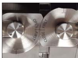
Valve handle locking system
