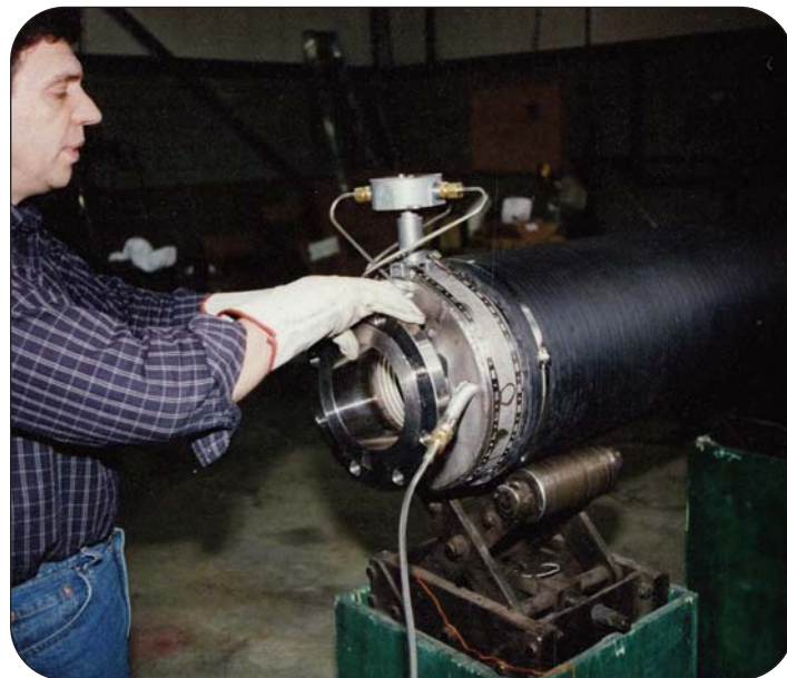
Manufacturing Sure-Temp™ electrically heated hose assembly
