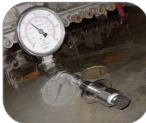
Pneumatic test at 100 psi
