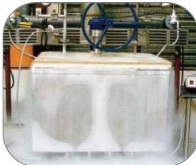
Cryogenic test bench at -320°F
