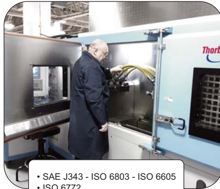
Flex-impulse testing up to 700 BAR @ 150°C
