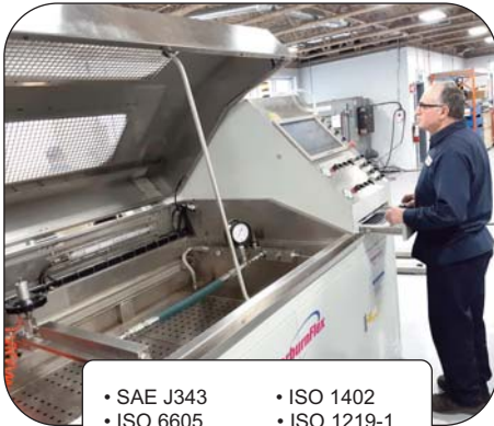
Proof testing up to 6 hoses 1000 BAR
