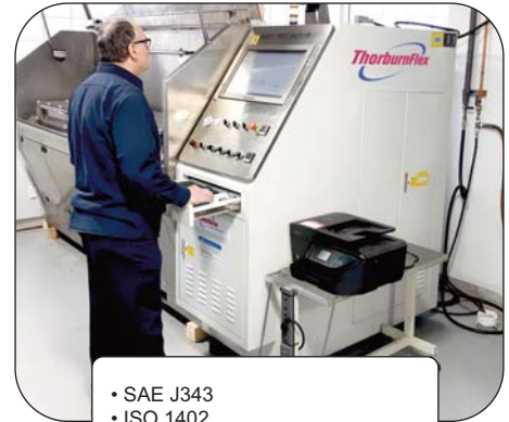
Burst testing up to 4000 BAR
