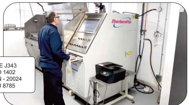
Burst testing up to 4000 BAR
