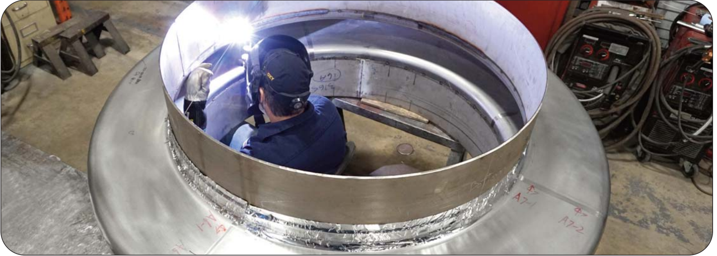
Welding a Thorburn Series AFU Inconel 625 250mm height single convolution bellows expansion joint without crest weld
