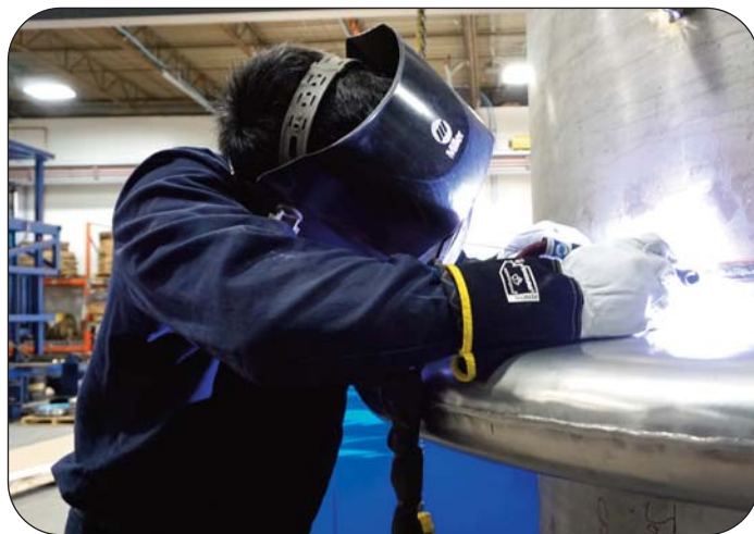
Welding a Thorburn Series AFS single convolution lens High-Core bellows
