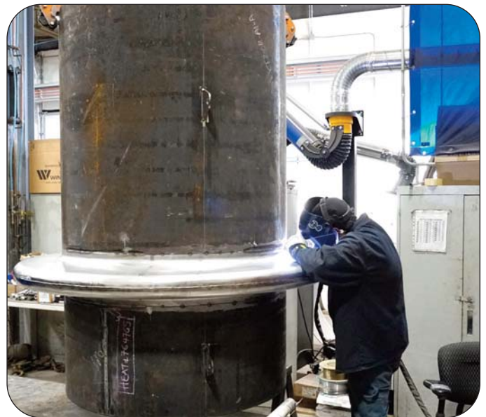
Manufacturing a Thorburn Series AFS single convolution lens High-Core bellows
